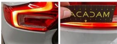
Reflector, Crack, Replace
