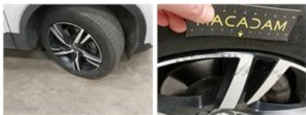
Alloy rim RR polished, Scratch(es), Repair and paint (complete)
