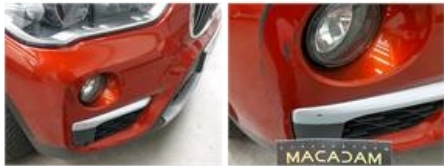
Bumper F, Scratch(es), Repair and paint (complete)
