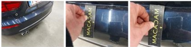
Wing RL, Scratch(es), Spot repair
