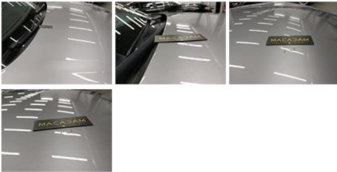
Roof, Hail damage, Paintless dent repair (hail)
